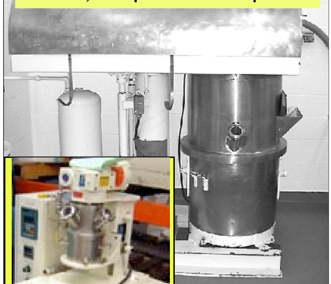
Ross HDM-40 Gallon, double planetary mixer, from pharmaceutical plant
